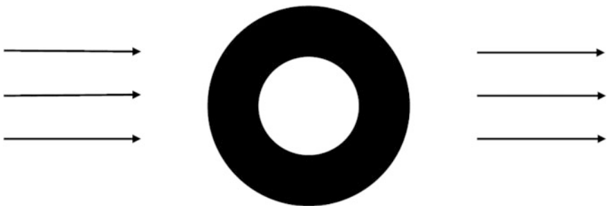
Fig. 1.5 Schematic of the application of a metamaterial in the form of a hollow cylinder to hide an object placed within the cylinder. Parallel rays of light incident from the left are sent through the system, exiting as parallel rays on the right of the system. The object within the cylinder is not evident in the light passing to the right of the cylinder
