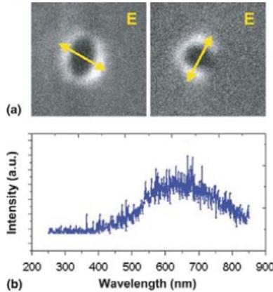
Figure 8.12. Electron-beam induced surface plasmon emission of light. (a) Cathodoluminescence image for two different polarizations. (b) Corresponding spectrum. Reprinted from [Degiron et al., 2004], copyright 2004, with permission from Elsevier.
