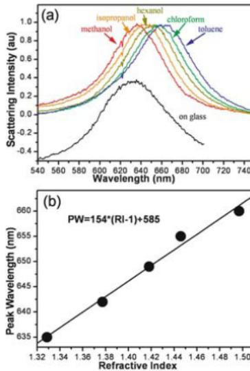
*Figure 10.11.* (a) Normalized scattering spectra of a single gold nanoparticle in various solvents measured through the fiber. (b) Dependence of the resonance position on the index of refraction of the solvent. Reprinted with permission from [Eah et al., 2005]. Copyright 2005, American Institute of Physics.
