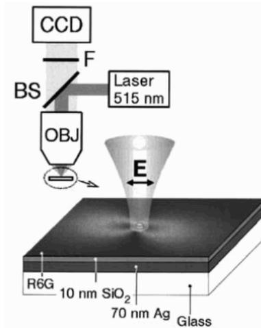
*Figure 4.3.* Fluorescence imaging of SPP fields. A SPP on a 70 nm silver film is excited via illumination of a nanoparticle (phase-matching via a defect) using a 100 $\times$  objective, and the field distribution of the mode imaged by detecting the fluorescent emission of a coating layer doped with Rhodamin 6G. Reprinted with permission from [Ditlbacher et al., 2002a]. Copyright 2002, American Institute of Physics.
