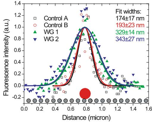
Figure 7.26. Intensity of the fluorescence signal along the cross-cuts indicated in Fig. 7.25c,d for control fluorescent spheres located away from waveguides (squares) and spheres located on top of particle waveguides (triangles). The increase in width of the fluorescence peaks for the latter is indicative of excitation at a distance via the particle waveguides (see sketch in Fig. 7.25a). Reprinted by permission of Macmillan Publishers Ltd: Nature Materials [Maier et al., 2003b], copyright 2003.
