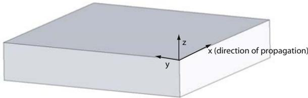
*Figure 2.1.* Definition of a planar waveguide geometry. The waves propagate along the x-direction in a cartesian coordinate system.
