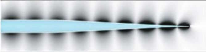
*Figure 7.19.* Distribution of the electric field around a tapered silica fiber coated with a silver layer of thickness 40 nm. The full taper angle is  $6^\circ$ , and the initial radius of the silica taper is 160 nm. The apex is terminated with a 10 nm semi-sphere. Transfer of energy from the fiber to the plasmon mode and energy concentration is visible ( $\lambda_0 = 1.3 \mu\text{m}$ ).
