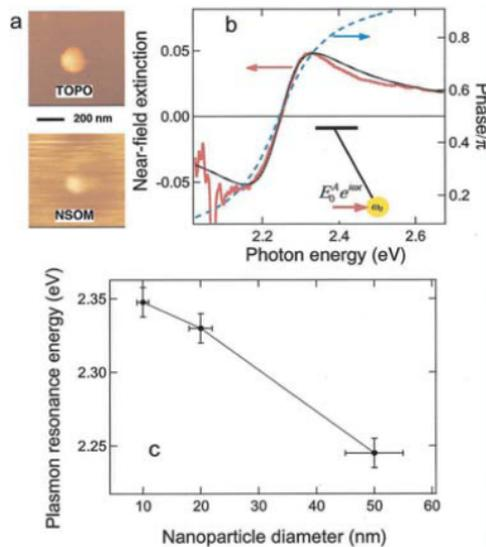
Figure 10.4. (a) Topography and near-field image of a 50 nm gold sphere. (b) Near-field extinction spectrum (solid gray curve) compared with interference (black curve) and phase (dashed curve) spectra for a single 50 nm gold particle calculated using a forced harmonic oscillator model. (c) Dependence of resonance frequency on particle size inferred from the spectra. Reprinted with permission from [Mikhailovsky et al., 2003]. Copyright 2003, Optical Society of America.
