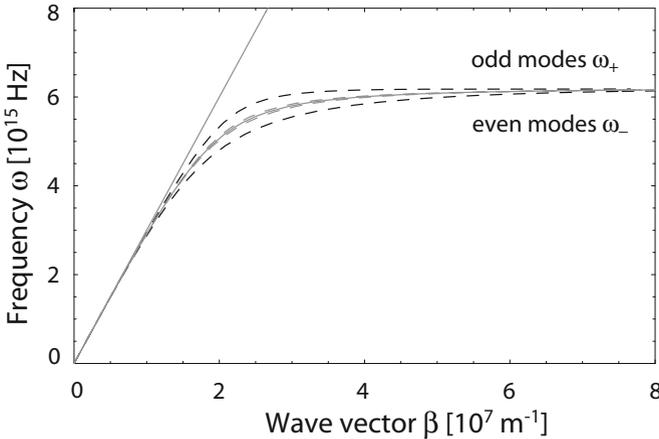
*Figure 2.6.* Dispersion relation of the coupled odd and even modes for an air/silver/air multilayer with a metal core of thickness 100 nm (dashed gray curves) and 50 nm (dashed black curves). Also shown is the dispersion of a single silver/air interface (gray curve). Silver is modeled as a Drude metal with negligible damping.
