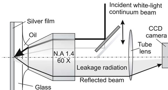
*Figure 3.9.* Schematic of the excitation of a white-light continuum of SPPs and their observation via detection of the leakage radiation using an index-matched oil immersion lens. Reprinted with permission from [Bouhelier and Wiederrecht, 2005]. Copyright 2005 by the Optical Society of America.
