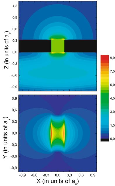
*Figure 8.14.* Enhancement of the electric field  $|E|$  with respect to the incident field for a rectangular aperture of Fig. 8.13 with  $a_y/a_x = 3$  and  $h = a_y/3$  at the resonant wavelength. The top panel shows a cut through the center of the aperture, and the lower panel the field distribution at the entrance surface. Reprinted with permission from [García-Vidal et al., 2005b]. Copyright 2005 by the American Physical Society.
