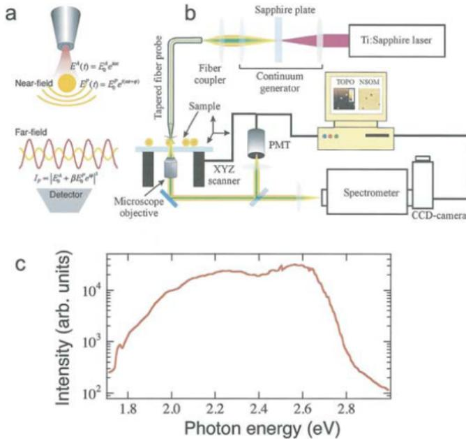
*Figure 10.3.* Sketch of excitation geometry (a) and experimental setup (b) for white-light illumination mode near-field optical microscopy. (c) Spectrum of the white light supercontinuum at the output of the fiber tip. Reprinted with permission from [Mikhailovsky et al., 2003]. Copyright 2003, Optical Society of America.
