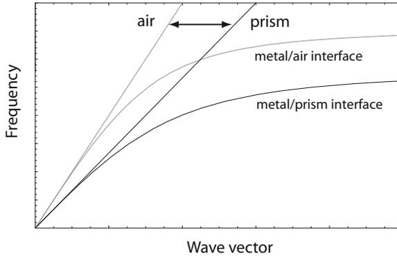
*Figure 3.5.* Prism coupling and SPP dispersion. Only propagation constants between the light lines of air and the prism (usually glass) are accessible, resulting in additional SPP damping due to leakage radiation into the latter: the excited SPPs have propagation constants *inside* the prism light cone.
