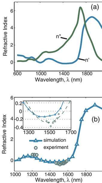
Figure 11.3. (a) Real and imaginary parts  $n'$ ,  $n''$  of the refractive index for the metamaterial of Fig. 11.2 determined using simulations. (b) Comparison between simulations (triangles) and experimentally determined values (circles) of the real part of the refractive index. The inset shows a magnified view of the region of negative refractive index. Copyright with permission from [Shalaev et al., 2005]. Copyright 2005, Optical Society of America.
