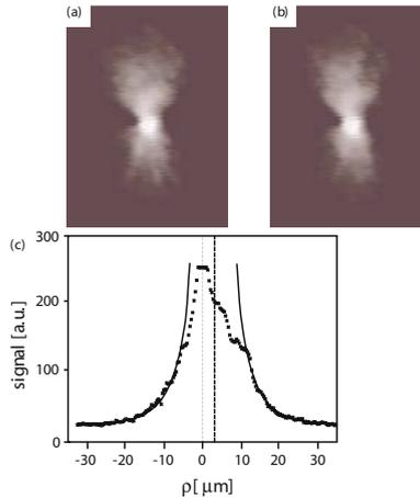
*Figure 3.13.* Spatial intensity distribution of SPPs on a silver film at  $\lambda = 633$  nm. (a), (b) are  $50\mu\text{m} \times 70\mu\text{m}$  images collected in the far field corresponding to two different locations of the exciting near-field probe. (c) Cross section through the intensity profile along the main symmetry axes of the spots and analytical fit using (3.4). Reprinted with permission from [Hecht et al., 1996]. Copyright 1996 by the American Physical Society.
