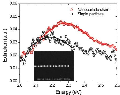
*Figure 7.24.* Experimentally observed plasmon resonance for single silver rods and a chain of closely-spaced rods under transverse illumination (along the long axis of the rods). The blue-shift between the two spectra is due to near-field interactions between particles in the chain. Reprinted by permission of Macmillan Publishers Ltd: Nature Materials [Maier et al., 2003b], copyright 2003.
