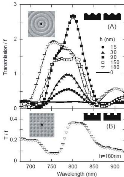
Figure 8.4. Transmission through a single circular aperture ( $d = 440$  nm) surrounded by concentric rings with sinusoidal cross section (A) or a square array of dimples (B) of height  $h$  milled into a 430 nm thick Ag/NiAg screen. Reprinted with permission from [Thio et al., 2001]. Copyright 2001, Optical Society of America.
