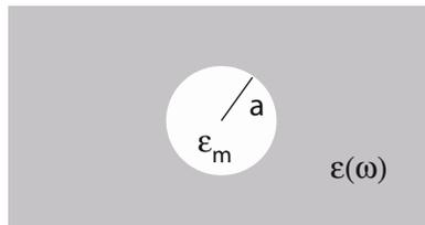
Figure 5.14. Spherical dielectric inclusion in a homogeneous metal.
