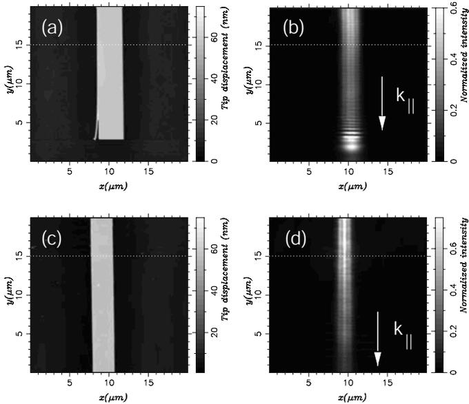
Figure 7.15. AFM (a and c) and near-field optical (b and d) images of gold stripes of height 55 nm and width  $w = 3.5 \mu\text{m}$  (a and b) or  $w = 2.5 \mu\text{m}$  (c and d). Reprinted with permission from [Weeber et al., 2003]. Copyright 2003 by the American Physical Society.
