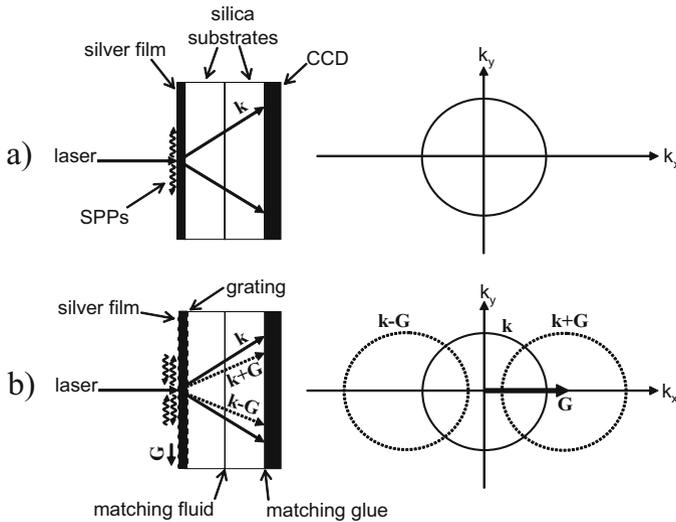
*Figure 4.8.* Experimental geometry of leakage radiation imaging for the determination of the SPP dispersion relation. (a) Planar silver surface: a single cone of light is emitted into the silica substrate. (b) Corrugated silver surface: the central cone is now intersected by other light cones due to SPPs scattered by the grating with Bragg vector  $\mathbf{G}$ . Reproduced with permission from [Giannattasio and Barnes, 2005]. Copyright 2005, Optical Society of America.
