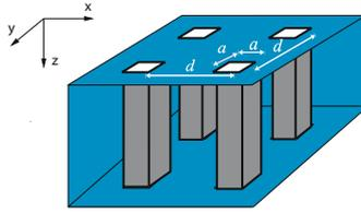
Figure 6.7. Two-dimensional square lattice of square holes of size  $a$  with lattice constant  $d$  in a semi-infinite perfect conductor. Reprinted with permission from [García-Vidal et al., 2005a]. Copyright 2005, Institute of Physics.
