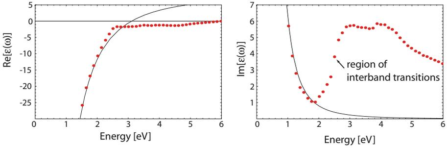
Figure 1.1. Dielectric function  $\varepsilon(\omega)$  (1.27) of the free electron gas (solid line) fitted to the literature values of the dielectric data for gold [Johnson and Christy, 1972] (dots). Interband transitions limit the validity of this model at visible and higher frequencies.
