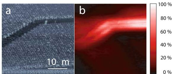
*Figure 7.8.* Topographical (a) and near-field optical (b) image of a channel defect waveguide in a triangular lattice of period 950 nm consisting of 438 nm wide and 80 nm high gold scatters on an gold film. A SPP excited at  $\lambda_0 = 1515$  nm incident from the right propagates through the channel. Reprinted with permission from [Marquart et al., 2005]. Copyright 2005, Optical Society of America.
