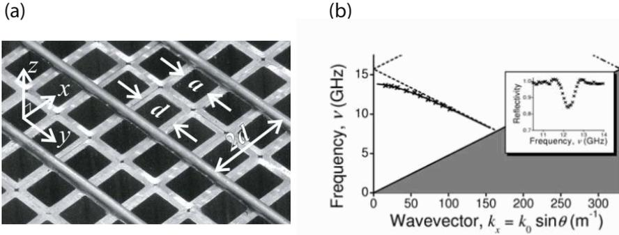
Figure 6.10. (a) Photograph of a two-dimensional array of hollow square brass tubes with side length  $d = 9.525$  mm, inner dimension  $a = 6.960$  mm and depth  $h = 45$  mm covered with a one-dimensional array of cylindrical rods used for diffractive coupling and zone-folding. (b) Dispersion relation of the surface mode obtained via the angle-dependence of the reflectivity dips (see inset). Reprinted with permission from [Hibbins et al., 2005]. Copyright 2005, AAAS.
