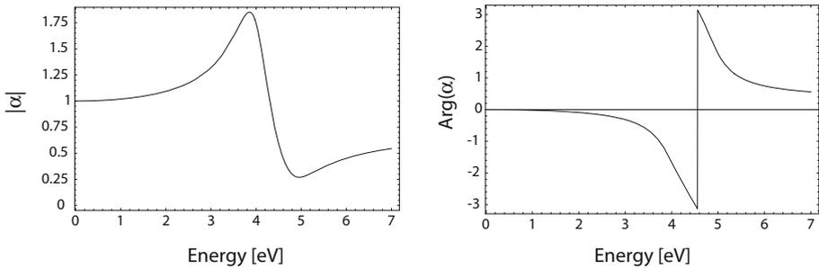
Figure 5.2. Absolute value and phase of the polarizability  $\alpha$  (5.7) of a sub-wavelength metal nanoparticle with respect to the frequency of the driving field (expressed in eV units). Here,  $\varepsilon(\omega)$  is taken as a Drude fit to the dielectric function of silver [Johnson and Christy, 1972].
