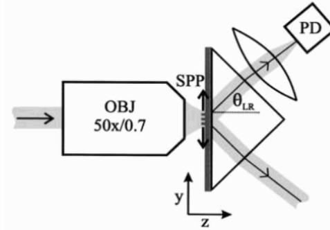
*Figure 4.6.* Experimental setup for leakage radiation imaging of SPP fields. Here, SPPs are excited using grating coupling, and the ensuing leakage radiation into the underlying prism collected using a photodiode. Reprinted with permission from [Ditlbacher et al., 2003]. Copyright 2003, American Institute of Physics.
