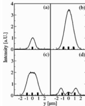
*Figure 4.7.* Quantifying coupling efficiency of a finite metal grating via collection of leakage radiation. The graphs show the experimentally observed distribution of leakage radiation vs. sample position (Fig. 4.6) for a single-ridge sample (a) and samples with three ridges of different lattice constants (b-d). The maximum intensity profile in (a) was normalized to 1. Reprinted with permission from [Ditlbacher et al., 2003]. Copyright 2003, American Institute of Physics.
