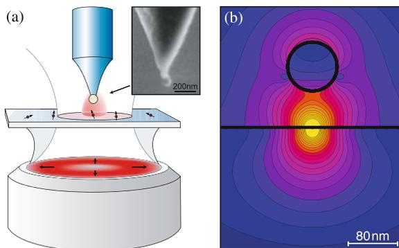
Figure 9.9. Experimental setup (a) and calculated field distribution for an emitter located on a glass substrate at a distance  $z = 60$  nm below a gold particle (b) for the study of single-molecule fluorescence near a gold sphere. Reprinted with permission from [Anger et al., 2006]. Copyright 2006 by the American Physical Society.
