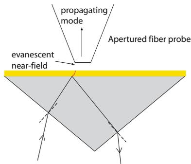
*Figure 4.1.* A typical setup for near-field optical imaging of SPP fields at a metal/air interface. The evanescent tail of the fields penetrating into the air is coupled to propagating modes in a tapered optical fiber tip. The SPPs can for example be excited via prism coupling (shown), a tightly focused beam, or particle impact.
