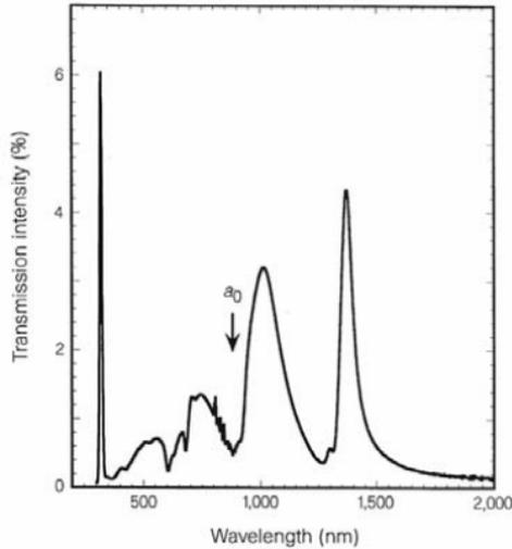
Figure 8.2. Normal-incidence transmission spectrum for a silver screen perforated with a square array of holes of diameter  $d = 150$  nm and lattice constant  $a_0 = 900$  nm. The thickness of the screen is 200 nm. Reprinted by permission from Macmillan Publishers Ltd: Nature [Ebbesen et al., 1998], copyright 1998.
