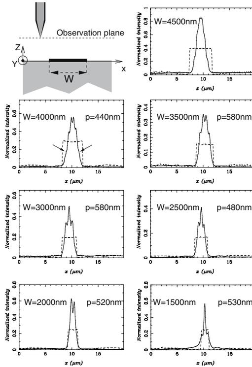
Figure 7.16. Cross-cuts through the near-field intensity of various stripes of width  $w$  (see Fig. 7.15).  $p$  denotes the distance between the peaks. Compare with the calculated profiles in the third column of Fig. 7.13. Reprinted with permission from [Weeber et al., 2003]. Copyright 2003 by the American Physical Society.
