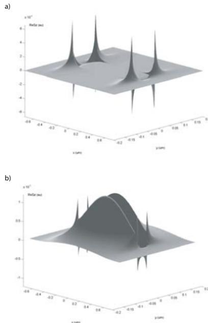
*Figure 7.11.* Mode profile of the real part of the Poynting vector for the long-ranging  $ss_b^0$  mode at  $\lambda_0 = 633$  nm of a 100 nm (a) or 40 nm (b) thick and  $1 \mu\text{m}$  wide silver stripe, showing the Gaussian-like mode shape for small film thickness. Reprinted with permission from [Berini, 1999]. Copyright 1999, Optical Society of America.
