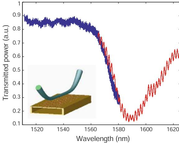
*Figure 3.14.* Excitation of SPPs propagating on a metal nanoparticle plasmon waveguide situated on a thin silicon membrane using a fiber taper (sketch in inset). The transmission spectrum shows the power transmitted through the taper past the coupling region, demonstrating a power transfer efficiency of 75% at  $\lambda_0 = 1590$  nm due to phase-matching. Reprinted with permission from [Maier et al., 2005]. Copyright 2005, American Institute of Physics.
