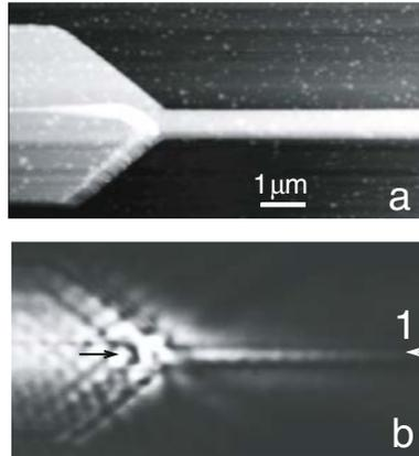
*Figure 7.17.* Topography (a) and optical near-field intensity (b) of a  $20\ \mu\text{m}$  long gold nanowire of width  $w = 200\ \text{nm}$  excited at  $\lambda_0 = 800\ \text{nm}$ . The arrows mark the position of data-cut 1 shown in Fig. 7.18. Reproduced with permission from [Krenn et al., 2002]. Copyright 2002, Institute of Physics.
