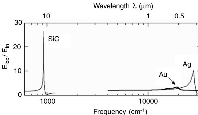
*Figure 6.11.* Calculated field enhancement of the polarizability of a 10 nm SiC sphere at the Fröhlich frequency defined by (5.8), compared to spheres consisting of gold or silver. Reprinted by permission from McMillan Publishers Ltd: Nature [Hillenbrand et al., 2002], copyright 2002.
