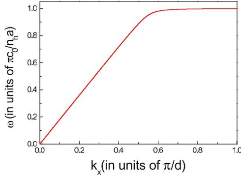
Figure 6.8. Dispersion relation (6.9) of the SPP-like bound mode at the interface between a perforated perfect conductor and vacuum for  $a/d = 0.6$  and  $\epsilon_h = 9$ . Reprinted with permission from [García-Vidal et al., 2005a]. Copyright 2005, Institute of Physics.
