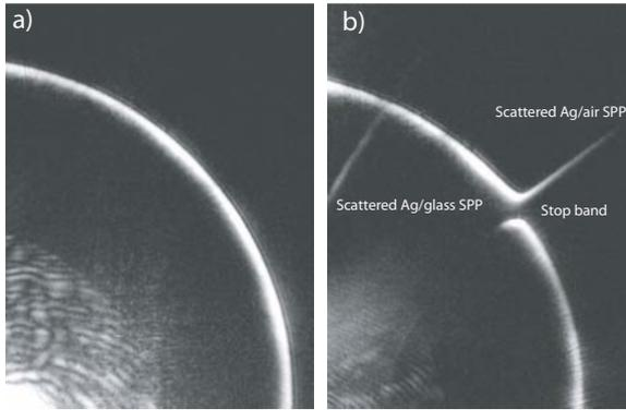
Figure 4.9. Direct image of the conical radiation in  $k$ -space sketched in Fig. 4.8 recorded by a CCD array. (a) Planar sample. (b) Imaging of the stop band emerging at the intersection between the two cones in  $k$ -space. Reproduced with permission from [Giannattasio and Barnes, 2005]. Copyright 2005, Optical Society of America.
