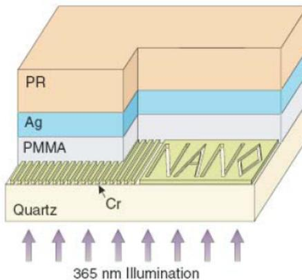
*Figure 11.5.* Schematic of an optical superlens. A 35 nm thin silver imaging layer is separated from a chrome mask via a 40 nm polymer layer. Upon illumination of the chrome mask with UV light, an image mediated by the silver layer is recorded in a thin photoresist film. Reprinted with permission from [Fang et al., 2005]. Copyright 2005, AAAS.
