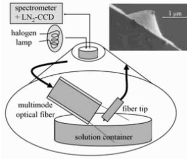
*Figure 10.10.* Optical setup for measuring the scattering of a single nanoparticle in various solvents through an optical fiber. The inset shows a SEM image of a nanoparticle attached to the fiber tip. Reprinted with permission from [Eah et al., 2005]. Copyright 2005, American Institute of Physics.
