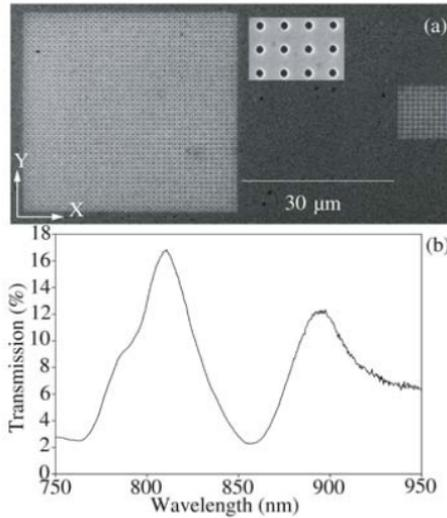
*Figure 3.7.* (a) SEM image of two microhole arrays with period 760 nm and hole diameter 250 nm separated by 30  $\mu\text{m}$  used for sourcing (right array) and probing (left array) of SPPs. The inset shows a close-up of individual holes. (b) Normal-incidence white light transmission spectrum of the arrays. Reprinted with permission from [Devaux et al., 2003]. Copyright 2003, American Institute of Physics.
