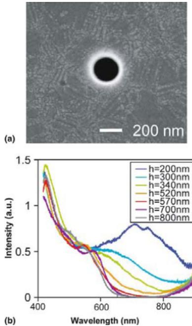
*Figure 8.11.* Transmission of light through a single sub-wavelength hole milled into a free-standing silver film (a). The transmission peak for small screen thickness  $h$  (b) is due to localized surface plasmons. Reprinted from [Degiron et al., 2004], copyright 2004, with permission from Elsevier.
