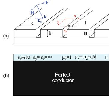
Figure 6.4. (a) One-dimensional array of grooves of width  $a$  and depth  $h$  with lattice constant  $d$ . (b) The effective medium approximation of the structure. Reprinted with permission from [García-Vidal et al., 2005a]. Copyright 2005, Institute of Physics.
