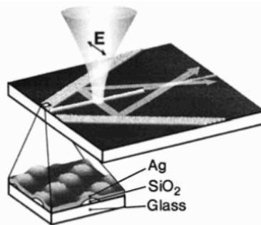
*Figure 7.1.* Routing of SPPs on a planar silver film using surface modulations. A laser beam focused on a nanowire or nanoparticle defect for phase-matching acts as a local source for SPPs. The micrograph shows a Bragg reflector consisting of lines of regularly spaced, particle-like undulations (Fig. 7.2). Reprinted with permission from [Ditlbacher et al., 2002b]. Copyright 2002, American Institute of Physics.
