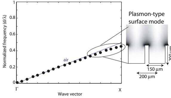
Figure 6.9. Dispersion relation of the SPP-like mode of a perfect conductor perforated with square holes of side  $a = 150\mu\text{m}$  and depth  $h = 200\mu\text{m}$  arranged on a square lattice with lattice constant  $d = 200\mu\text{m}$ . The distribution of the electric field at the band edge is also shown.
