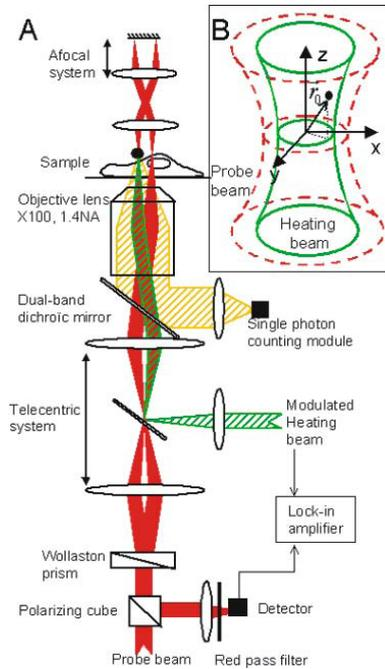
*Figure 10.7.* Experimental setup for photothermal imaging of very small nanoparticles. For a description see main text. Reprinted with permission from [Cognet et al., 2003]. Copyright 2003, National Academy of Sciences, U.S.A.
