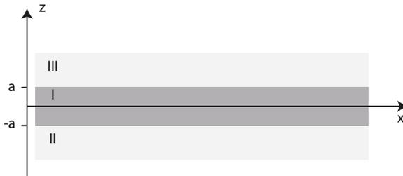
Figure 2.5. Geometry of a three-layer system consisting of a thin layer I sandwiched between two infinite half spaces II and III.
