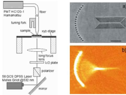
*Figure 7.5.* Experimental setup of the excitation and near-field imaging for SPP focusing on a holey metal film (left). (a) SEM and (b) near-field optical image of the nanohole focusing array which couples the launched SPPs into a 250 nm wide silver stripe guide. Reprinted with permission from [Yin et al., 2005]. Copyright 2005, American Chemical Society.
