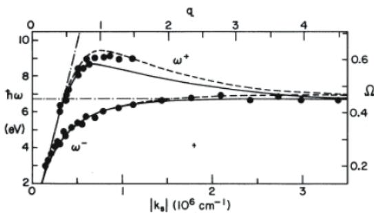
*Figure 3.3.* Comparison of the experimental data presented in Fig. 3.2(dots) with the theoretical dispersion curves of the two coupled modes. For the theoretical analysis see Fig. 2.6. For the calculations, the aluminum film has been assumed to be embedded into amorphous alumina (dashed curves) or alumina in its  $\alpha$ -phase (continuous curves). Reprinted with permission from [Pettit et al., 1975]. Copyright 1975 by the American Physical Society.
