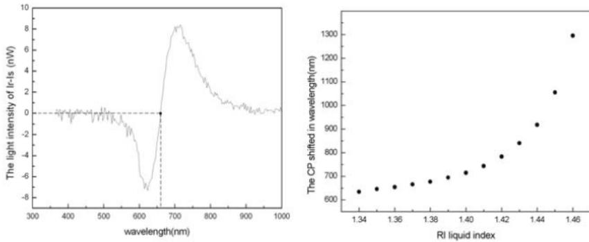
*Figure 10.15.* (a) Difference in light intensity between the sensing and the reference arm vs. optical wavelength using the SPP fiber sensor structure of Fig. 10.14. Here, the sensing arm is immersed in alcohol, and the reference fiber in distilled water. (b) Experimental results for the shift in crossing-point wavelength of the two SPP spectra versus refractive index. Reprinted with permission from [Tsai et al., 2005]. Copyright 2005, Optical Society of America.
