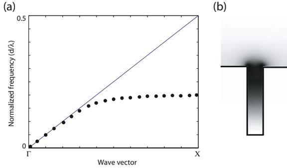
Figure 6.6. Dispersion relation (a) and electric field distribution in the unit cell at the band edge (b) for a SPP-like surface mode for  $h = d = 50\mu\text{m}$  and  $a = 10\mu$  calculated using finite-difference time-domain simulations.
