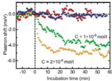
*Figure 10.6.* Resonance shift versus incubation time for streptavidin-BSA binding for different streptavidin concentrations  $C$  added at  $t = 0$ , and control experiments. Reprinted with permission from [Raschke et al., 2003]. Copyright 2003, American Chemical Society.
