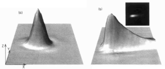
*Figure 4.2.* Near-field image of a HeNe laser beam ( $\lambda = 633$  nm) internally incident on an uncoated (a) prism face and a prism face coated with a 53 nm thick silver film (b) at an angle greater than the critical angle (scan range  $40 \times 40 \mu\text{m}$ ). The exponentially decaying tail in (b) is due to SPP propagation away from the excitation region. Reprinted with permission from [Dawson et al., 1994]. Copyright 1994 by the American Physical Society.
