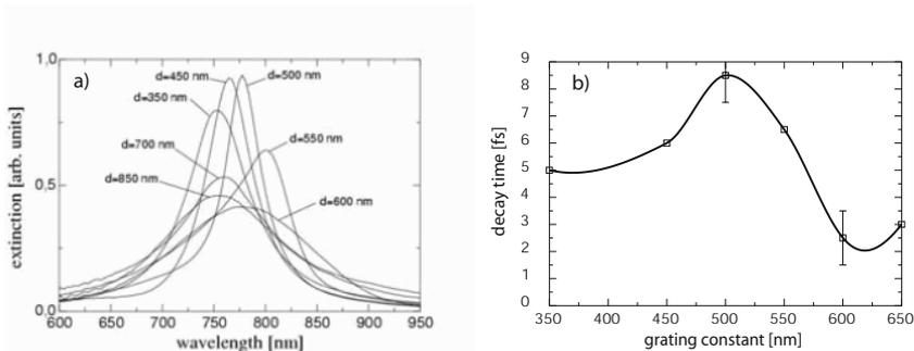
*Figure 5.13.* (a) Extinction spectra for square two-dimensional gratings of gold nanoparticles (height 14 nm, diameter 150 nm) with grating constant  $d$  situated on a glass substrate. (b) Plasmon decay time versus grating constant observed using a time-resolved measurement. The solid curve is a guide to the eye. Reproduced with permission from [Lamprecht et al., 2000]. Copyright 2000 by the American Physical Society.
