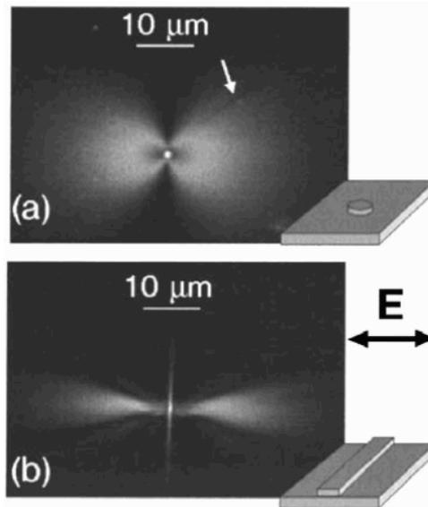
*Figure 4.4.* Fluorescence images of the intensity distribution of SPPs excited by illumination of (a) a silver nanoparticle (diameter 200 nm, height 60 nm), and (b) a silver nanowire (width 200 nm, height 60 nm, length  $20\ \mu\text{m}$ ). The particles are situated on a continuous silver film supporting SPPs. Reprinted with permission from [Ditlbacher et al., 2002a]. Copyright 2002, American Institute of Physics.
