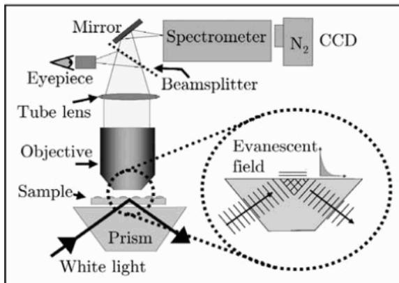
*Figure 10.1.* Setup for single-particle spectroscopy using evanescent excitation via total internal reflection at a prism and the monitoring of scattered light. Reprinted with permission from [Sönnichsen et al., 2000]. Copyright 2000, American Institute of Physics.
