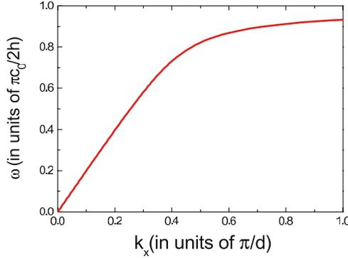
Figure 6.5. Dispersion relation (6.4) of the SPP-like mode of a groove array for the case  $a/d = 0.2$  and  $h = d$ . Reprinted with permission from [García-Vidal et al., 2005a]. Copyright 2005, Institute of Physics.
