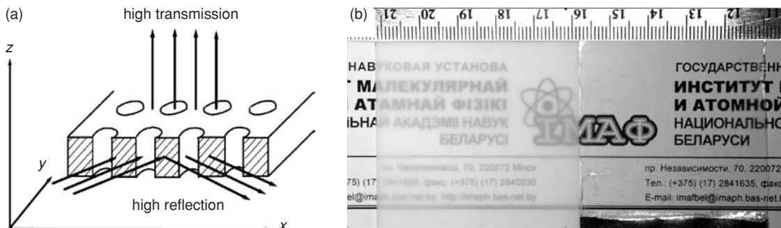
Fig. 7.27 High transparency of a two-dimensionally periodic dielectric slab in the direction along the pore axis. (a) A sketch of high reflection and high transmission directions. (b) Imaging through an opaque polymer film (left) and through a nanoporous alumina slab (right) with size 5 cm \times 5 cm. Note the residual piece of aluminium foil in the bottom of the alumina slab.
