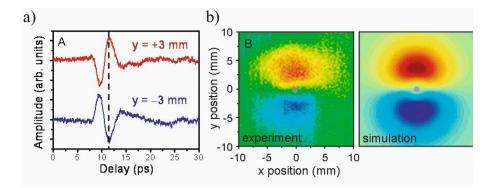
*Figure 6.3.* THz SPP propagation on a bare stainless-steel wire. a) Time-domain electric field waveform 3 mm above and below the wire. b) Experimental and simulated spatial mode profile. The radial nature of the mode is evident. Reprinted with permission from Macmillan Publishers Ltd: Nature [Wang and Mittleman, 2005], copyright 2004.
