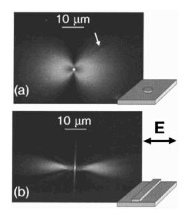
*Figure 4.4.* Fluorescence images of the intensity distribution of SPPs excited by illumination of (a) a silver nanoparticle (diameter 200 nm, height 60 nm), and (b) a silver nanowire (width 200 nm, height 60 nm, length 20  $\mu$ m). The particles are situated on a continuous silver film supporting SPPs. Reprinted with permission from [Ditlbacher et al., 2002a]. Copyright 2002, American Institute of Physics.
