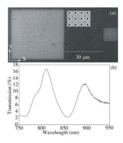
*Figure 3.7.* (a) SEM image of two microhole arrays with period 760 nm and hole diameter 250 nm separated by 30  $\mu$ m used for sourcing (right array) and probing (left array) of SPPs. The inset shows a close-up of individual holes. (b) Normal-incidence white light transmission spectrum of the arrays. Reprinted with permission from [Devaux et al., 2003]. Copyright 2003, American Institute of Physics.
