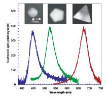
*Figure 5.7.* Scattering spectra of single silver nanoparticles of different shapes obtained in dark-field configuration. Reprinted with permission from [Mock et al., 2002a]. Copyright 2002, American Institute of Physics.
