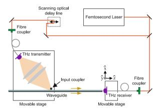
*Figure 6.2.* Typical setup for the generation and detection of broadband THz pulses. Input coupling to SPPs is achieved using scattering at a small gap between the guiding structure and a sharp edge. Reprinted with permission from Macmillan Publishers Ltd: Nature [Wang and Mittleman, 2005], copyright 2004.
