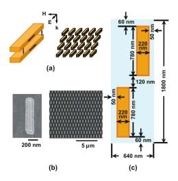
*Figure 11.2.* (a) Schematic and (b) SEM image of a planar metamaterial consisting of pairs of parallel gold nanorods. (c) Sketch of the unit cell of this structure. Reprinted with permission from [Shalaev et al., 2005]. Copyright 2005, Optical Society of America.
