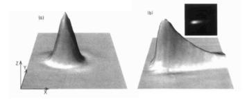
*Figure 4.2.* Near-field image of a HeNe laser beam ( $\lambda = 633$  nm) internally incident on an uncoated (a) prism face and a prism face coated with a 53 nm thick silver film (b) at an angle greater than the critical angle (scan range 40x40  $\mu$ m). The exponentially decaying tail in (b) is due to SPP propagation away from the excitation region. Reprinted with permission from [Dawson et al., 1994]. Copyright 1994 by the American Physical Society.
