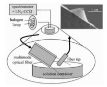
*Figure 10.10.* Optical setup for measuring the scattering of a single nanoparticle in various solvents through an optical fiber. The inset shows a SEM image of a nanoparticle attached to the fiber tip. Reprinted with permission from [Eah et al., 2005]. Copyright 2005, American Institute of Physics.
