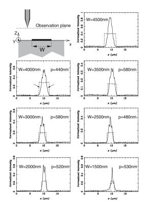
*Figure 7.16.* Cross-cuts through the near-field intensity of various stripes of width w (see Fig. 7.15). p denotes the distance between the peaks. Compare with the calculated profiles in the third column of Fig. 7.13. Reprinted with permission from [Weeber et al., 2003]. Copyright 2003 by the American Physical Society.
