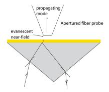
*Figure 4.1.* A typical setup for near-field optical imaging of SPP fields at a metal/air interface. The evanescent tail of the fields penetrating into the air is coupled to propagating modes in a tapered optical fiber tip. The SPPs can for example be excited via prism coupling (shown), a tightly focused beam, or particle impact.
