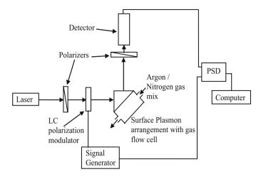
*Figure 10.12.* Experimental setup for differential ellipsometric detection of refractive index changes using SPPs on a metal film excited via prism coupling. Reprinted with permission [Hooper and Sambles, 2004b]. Copyright 2004, American Institute of Physics.
