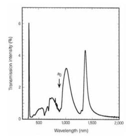
*Figure 8.2.* Normal-incidence transmission spectrum for a silver screen perforated with a square array of holes of diameter d = 150 nm and lattice constant  $a_0 = 900$  nm. The thickness of the screen is 200 nm. Reprinted by permission from Macmillan Publishers Ltd: Nature [Ebbesen et al., 1998], copyright 1998.
