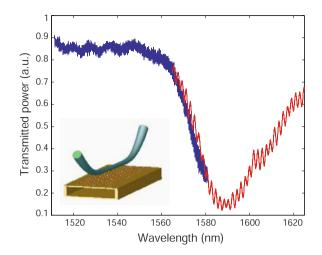
*Figure 3.14.* Excitation of SPPs propagating on a metal nanoparticle plasmon waveguide situated on a thin silicon membrane using a fiber taper (sketch in inset). The transmission spectrum shows the power transmitted through the taper past the coupling region, demonstrating a power transfer efficiency of 75% at  $\lambda_0 = 1590$  nm due to phase-matching. Reprinted with permission from [Maier et al., 2005]. Copyright 2005, American Institute of Physics.
