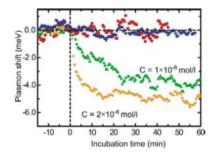
*Figure 10.6.* Resonance shift versus incubation time for streptavidin-BSA binding for different streptavidin concentrations *C* added at t = 0, and control experiments. Reprinted with permission from [Raschke et al., 2003]. Copyright 2003, American Chemical Society.
