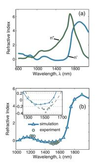
*Figure 11.3.* (a) Real and imaginary parts n', n'' of the refractive index for the metamaterial of Fig. 11.2 determined using simulations. (b) Comparison between simulations (triangles) and experimentally determined values (circles) of the real part of the refractive index. The inset shows a magnified view of the region of negative refractive index. Copyright with permission from [Shalaev et al., 2005]. Copyright 2005, Optical Society of America.
