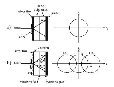
*Figure 4.8.* Experimental geometry of leakage radiation imaging for the determination of the SPP dispersion relation. (a) Planar silver surface: a single cone of light is emitted into the silica substrate. (b) Corrugated silver surface: the central cone is now intersected by other light cones due to SPPs scattered by the grating with Bragg vector **G**. Reproduced with permission from [Giannattasio and Barnes, 2005]. Copyright 2005, Optical Society of America.
