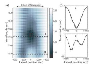
*Figure 7.28.* (a) Power transferred past the coupling region vs. wavelength and transverse taper position. Both the fundamental and the first-order mode are shown in data cuts (b). Reprinted with permission from [Maier et al., 2005]. Copyright 2005, American Institute of Physics.
