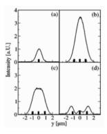
*Figure 4.7.* Quantifying coupling efficiency of a finite metal grating via collection of leakage radiation. The graphs show the experimentally observed distribution of leakage radiation vs. sample position (Fig. 4.6) for a single-ridge sample (a) and samples with three ridges of different lattice constants (b-d). The maximum intensity profile in (a) was normalized to 1. Reprinted with permission from [Ditlbacher et al., 2003]. Copyright 2003, American Institute of Physics.
