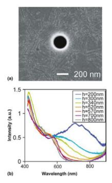
*Figure 8.11.* Transmission of light through a single sub-wavelength hole milled into a freestanding silver film (a). The transmission peak for small screen thickness h (b) is due to localized surface plasmons. Reprinted from [Degiron et al., 2004], copyright 2004, with permission from Elsevier.
