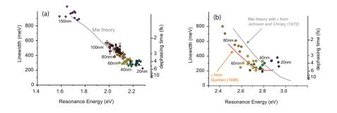
*Figure 5.5.* Linewidth of plasmon resonances of gold (a) and silver (b) nanospheres measured using dark-field microscopy, compared with predictions from Mie theory [Sönnichsen et al., 2002a]. Copyright 2002, Institute of Physics.
