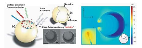
*Figure 9.5.* Fabrication process of crescent moon structures (left) and electric field profile (right) showing hot-spots at the tips of the moon structure. Reprinted with permission from [Lu et al., 2005]. Copyright 2005, American Chemical Society.
