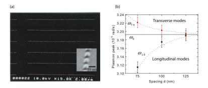
*Figure 5.11.* SEM image of arrays of closely spaced gold nanoparticles (a) and dependence of the spectral position of the dipole plasmon resonance on interparticle spacing (b). The dotted lines show a fit to the  $d^{-3}$  dependence of the coupling expected from a point-dipole model. Reprinted with permission from [Maier et al., 2002a]. Copyright 2002 by the American Physical Society.
