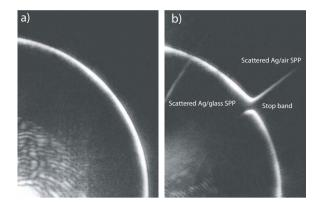
*Figure 4.9.* Direct image of the conical radiation in *k*-space sketched in Fig. 4.8 recorded by a CCD array. (a) Planar sample. (b) Imaging of the stop band emerging at the intersection between the two cones in *k*-space. Reproduced with permission from [Giannattasio and Barnes, 2005]. Copyright 2005, Optical Society of America.
