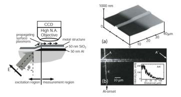
*Figure 7.12.* Prism coupling setup for the excitation of leaky SPPs propagating on thin metal stripes (left). The aluminum screen shields the stripe from direct excitation along its length. (a) AFM image of a 3  $\mu$ m wide stripe. (b) Scattered light image showing the propagating SPP excited at  $\lambda_0 = 633$  nm. Reprinted with permission from [Lamprecht et al., 2001]. Copyright 2001, American Institute of Physics.
