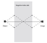
*Figure 11.4.* Schematic of the planar negative-index lens. Light diverging from a point source converges back towards a point in the negative-index medium due to negative refraction. On the other side of the planar slab, another focus is formed.
