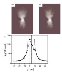
*Figure 3.13.* Spatial intensity distribution of SPPs on a silver film at  $\lambda = 633$  nm. (a), (b) are  $50\mu m \times 70\mu m$  images collected in the far field corresponding to two different locations of the exciting near-field probe. (c) Cross section through the intensity profile along the main symmetry axes of the spots and analytical fit using (3.4). Reprinted with permission from [Hecht et al., 1996]. Copyright 1996 by the American Physical Society.
