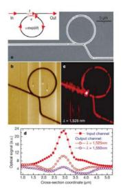
*Figure 7.21.* SEM (a), topographical (b) and near-field optical images (c) of a channel drop filter based on a V-groove waveguide and a ring resonator. Panel (d) shows normalized cross sections of the input and output channel obtained from (c) for two different wavelengths, demonstrating the extinction ratio on resonance. Reprinted by permission from Macmillan Publishers Ltd: Nature [Bozhevolnyi et al., 2006], copyright 2006.
