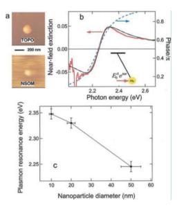
*Figure 10.4.* (a) Topography and near-field image of a 50 nm gold sphere. (b) Near-field extinction spectrum (solid gray curve) compared with interference (black curve) and phase (dashed curve) spectra for a single 50 nm gold particle calculated using a forced harmonic oscillator model. (c) Dependence of resonance frequency on particle size inferred from the spectra. Reprinted with permission from [Mikhailovsky et al., 2003]. Copyright 2003, Optical Society of America.
