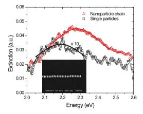
*Figure 7.24.* Experimentally observed plasmon resonance for single silver rods and a chain of closely-spaced rods under transverse illumination (along the long axis of the rods). The blue-shift between the two spectra is due to near-field interactions between particles in the chain. Reprinted by permission of Macmillan Publishers Ltd: Nature Materials [Maier et al., 2003b], copyright 2003.
