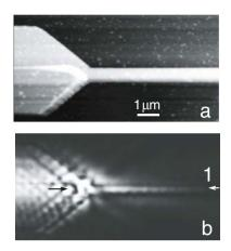
*Figure 7.17.* Topography (a) and optical near-field intensity (b) of a 20  $\mu$ m long gold nanowire of width w = 200 nm excited at  $\lambda_0 = 800$  nm. The arrows mark the position of data-cut 1 shown in Fig. 7.18. Reproduced with permission from [Krenn et al., 2002]. Copyright 2002, Institute of Physics.
