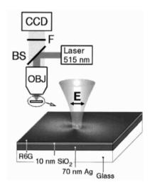
*Figure 4.3.* Fluorescence imaging of SPP fields. A SPP on a 70 nm silver film is excited via illumination of a nanoparticle (phase-matching via a defect) using a  $100 \times$  objective, and the field distribution of the mode imaged by detecting the fluorescent emission of a coating layer doped with Rhodamin 6G. Reprinted with permission from [Ditlbacher et al., 2002a]. Copyright 2002, American Institute of Physics.
