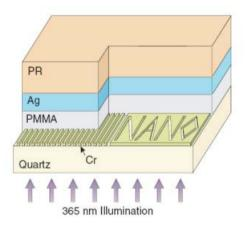
*Figure 11.5.* Schematic of an optical superlens. A 35 nm thin silver imaging layer is separated from a chrome mask via a 40 nm polymer layer. Upon illumination of the chrome mask with UV light, an image mediated by the silver layer is recorded in a thin photoresist film. Reprinted with permission from [Fang et al., 2005]. Copyright 2005, AAAS.
