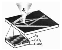
*Figure 7.1.* Routing of SPPs on a planar silver film using surface modulations. A laser beam focused on a nanowire or nanoparticle defect for phase-matching acts as a local source for SPPs. The micrograph shows a Bragg reflector consisting of lines of regularly spaced, particle-like undulations (Fig. 7.2). Reprinted with permission from [Ditlbacher et al., 2002b]. Copyright 2002, American Institute of Physics.
