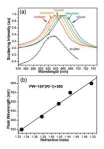
*Figure 10.11.* (a) Normalized scattering spectra of a single gold nanoparticle in various solvents measured through the fiber. (b) Dependence of the resonance position on the index of refraction of the solvent. Reprinted with permission from [Eah et al., 2005]. Copyright 2005, American Institute of Physics.
