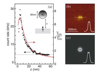
*Figure 9.10.* Experimentally determined emission rate (dots) and comparison with the theoretical curve of Fig. 9.8b) (a) and near-field image (b) of a fluorescent molecule near a gold sphere. A theoretical calculation of the emission intensity is shown in (c). Reprinted with permission from [Anger et al., 2006]. Copyright 2006 by the American Physical Society.
