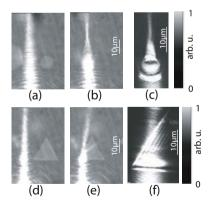
*Figure 7.4.* Focusing (top row) or reflection and refraction (bottom row) of SPPs via a cylindrical or triangular 40 nm thick dielectric structure deposited on top of a gold film. Images of the leakage radiation (a, b, d, e) and of the optical near field (e, f) clearly show the modification of SPP propagation for SPPs impinging on the dielectric structures (b, c, e, f). Reprinted with permission from [Hohenau et al., 2005b]. Copyright 2005, Optical Society of America.
