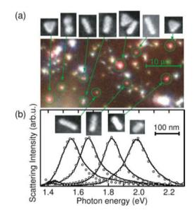
*Figure 5.8.* Optical dark field images together with SEM images of individual gold nanoparticles (a) and corresponding scattering spectra (b) for an incident light polarization along the long particle axis. Lines are experimental data, and circles cross sections calculated using the empirical formula (5.24). Reprinted with permission from [Kuwata et al., 2003]. Copyright 2003, American Institute of Physics.
