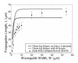
*Figure 7.13.* Comparison of experimental results (data points) for the SPP propagation length of thin silver stripes [Lamprecht et al., 2001] with numerical modeling of lowest-order, quasi-TM leaky modes (curves). Reprinted with permission from [Zia et al., 2005b]. Copyright 2005 by the American Physical Society.
