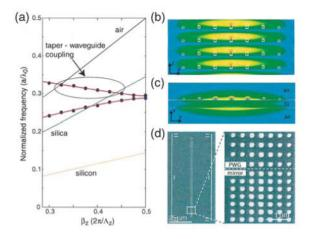
*Figure 7.27.* Dispersion relation (a) and mode profiles in top (b) and side (c) view of a metal nanoparticle plasmon waveguide on a thin Si membrane operating in the near-infrared. (d) SEM picture of a fabricated device. Reprinted with permission from [Maier et al., 2004]. Copyright 2004, American Institute of Physics.
