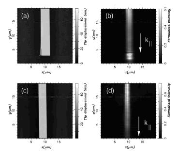
*Figure 7.15.* AFM (a and c) and near-field optical (b and d) images of gold stripes of height 55 nm and width  $w = 3.5 \ \mu m$  (a and b) or  $w = 2.5 \ \mu m$  (c and d). Reprinted with permission from [Weeber et al., 2003]. Copyright 2003 by the American Physical Society.
