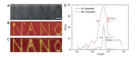
*Figure 11.6.* (a) FIB image of the object plane. The linewidth of the letters is about 40 nm. (b,c) AFM image of the developed photoresist with the silver imaging layer (Fig. 11.5) present (b) or replaced (c) by a PMMA layer. (d) Averaged cross section of the letter "A" with and without the lens. Reprinted with permission from [Fang et al., 2005]. Copyright 2005, AAAS.
