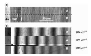
*Figure 6.14.* Topography (a) and near-field optical images (b) for surface phonon polariton propagation acquired using the setup of Fig. 6.13. Reprinted with permission from [Huber et al., 2005]. Copyright 2005, American Institute of Physics.
