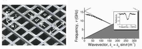
*Figure 6.10.* (a) Photograph of a two-dimensional array of hollow square brass tubes with side length d = 9.525 mm, inner dimension a = 6.960 mm and depth h = 45 mm covered with a one-dimensional array of cylindrical rods used for diffractive coupling and zone-folding. (b) Dispersion relation of the surface mode obtained via the angle-dependence of the reflectivity dips (see inset). Reprinted with permission from [Hibbins et al., 2005]. Copyright 2005, AAAS.
