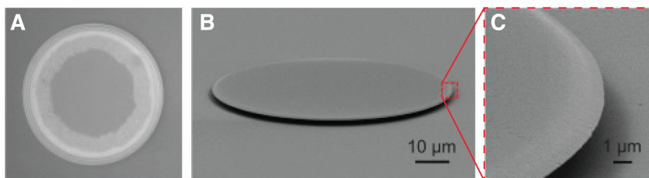
Figure 10: Microscope images of a typical LNOI microdisk resonator. (A) Optical microscope image of the microdisk from the top. (B) scanning electron microscope image showing the overview and (C) the edge of the microdisk. Reprinted with permission from Wang et al. [51]. © The Optical Society.
