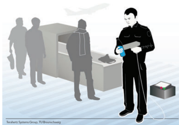
Figure 30 (online color at: www.lpr-journal.org ) Cartoon that illustrates the use of a handheld THz scanner for the analysis of bottles carried by passengers.
