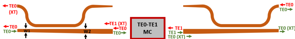
Fig. 2. Schematic of the circuit block for device characterization, showing the forward (in green) and reverse (in red) propagation through the TE 0 -TE 1 mode converter.
