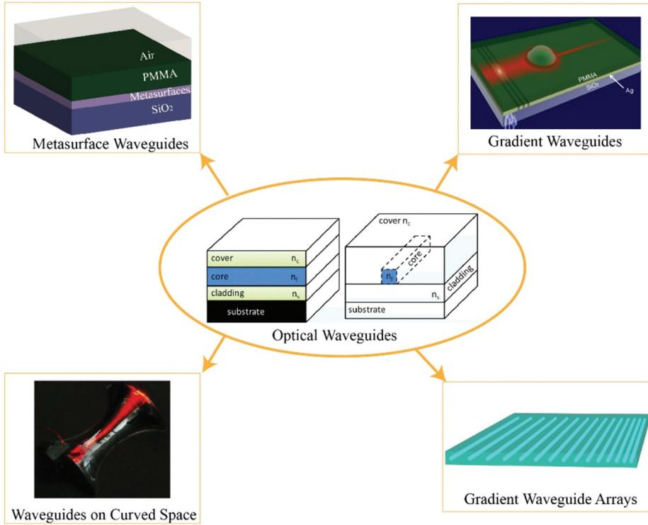
**Figure 1.** Different type waveguides for optical simulations inspired by general relativity.
