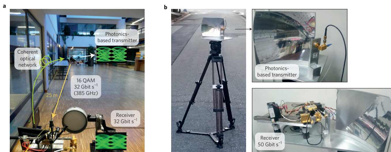
Figure 3 | Examples of THz links using photonics-based transmitters. a , Multi-level 32 Gbit s -1 link over 25 m with 16 QAM modulation delivered by a fibre-optic network. b , Real-time 50 Gbit s -1 link over 100 m with OOK modulation.
