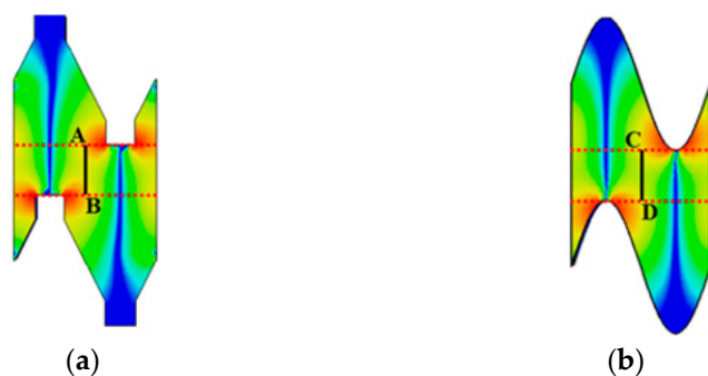
Figure 7. Distribution of E_z in the y - o - z plane of (a) SDSG-SWS, (b) SW-SWS at 340 GHz.
