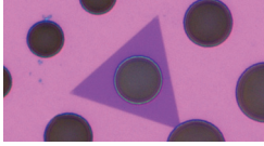
Optical image of the surface of suspended bilayer WS_2 on a holey SiO_2/Si substrate. Selected for an Editors' Suggestion. [Y. Xu et al. , Phys. Rev. Lett. 134 , 066904 (2025)]
