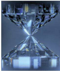
Diamond anvils used for studying iron-helium reactions under high pressures that occurred during the formation of Earth's core. Selected for a Synopsis in *Physics Magazine* and for an Editors' Suggestion. [T. Haruki *et al.*, Phys. Rev. Lett. **134**, 084101 (2025)]
