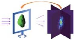
Schematics of a reconstruction process utilizing a phase retrieval algorithm in a 3D coherent x-ray diffraction imaging setup, where x-rays are scattered from a rotating sample to form patterns. [Fangzhou Ai, Oleg Shpyrko, and Vitaliy Lomakin, *Phys. Rev. Lett.* **134**, 236202 (2025)]
