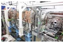
Experimental setup for muon acceleration showing accelerating cavity (left) and cooling chamber (right). Selected for a Viewpoint in *Physics Magazine* and for an Editors' Suggestion. [S. Aritome *et al.*, Phys. Rev. Lett. **134**, 245001 (2025)]
