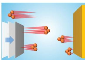
Controllable, 100- $\mu\text{m}$ -sized, tabletop Fermi accelerator in which ultracold atoms are accelerated by moving barriers: One of the walls moving toward the opposite wall causes bouncing atoms to gain energy. Selected for a Focus in *Physics Magazine* and for an Editors' Suggestion. [G. Barontini *et al.*, Phys. Rev. Lett. **135**, 025201 (2025)]
