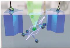
A nickel vacancy defect in diamond is located between two boron-implanted regions (blue) that are electrically contacted to form a junction for charge state control. The defect is optically addressed by a laser.
