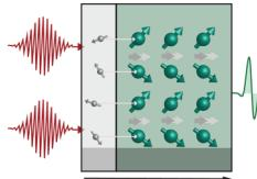
Schematic of a platinum-nickel oxide heterostructure emitting terahertz radiation (green line) in response to laser excitation (red arrows) in the presence of a magnetic field (black arrow). Selected for an Editors' Suggestion. [T. W. J. Metzger *et al.*, Phys. Rev. Lett. **135**, 076702 (2025)]
