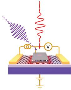
Schematic of a graphene spin field-effect junction device, measured by a femtosecond pump (purple arrow) probe (red arrow) technique. Selected for an Editors' Suggestion. [D. Muradas-Belinchón *et al.*, Phys. Rev. Lett. **135**, 097001 (2025)]
