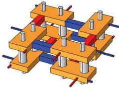
Unit cell of a three-dimensional acoustic lattice composed of resonators (orange) connected by coupling tubes (red, blue, and gray). Selected for an Editors' Suggestion. [H. T. Teo *et al.*, Phys. Rev. Lett. **135**, 136602 (2025)]
