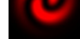
Intensity distributions for the superposition of Bessel-Gauss beams at a transverse plane at z = 0.75 m. For more, see the paper by Jkome-Silva et al., pp. 2760-2763.
